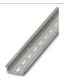
DIN rail, material: steel galvanized and passivated with a thick layer, perforated, height 7.5 mm, width 35 mm, length: 755 mm
