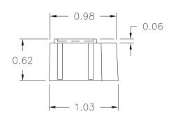
USE # 28 DRILL (0.140), #8-32 TAP, # 8-32 THREAD X 1/4 LG. CUP POITED, SLOTTED TYPE, SET SCREW 10357. -
