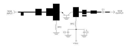
DIELECTRIC = 10 MIL THICK DUROID, Er = 2.3 C1, C2 = 82pF CHIP ATC "A" C3 = 100MFD @ 35V RFC = 5 turns #22 wire 1/16" I.D.
