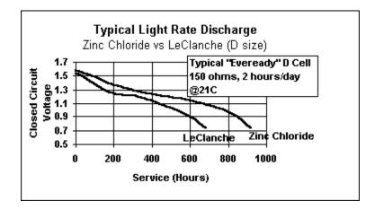
As the drain is increased, the service difference between Alkaline, Zinc Chloride and LeClanche systems increases. This relationship is shown by the following discharge curves. Typical carbon zinc moderate drain is defined as a current that would discharge the cell within 10-50 hours of use at room temperature.
