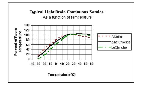
**Light Drain** is defined as a current that would discharge the battery after 50 or more hours of use at room temperature.
