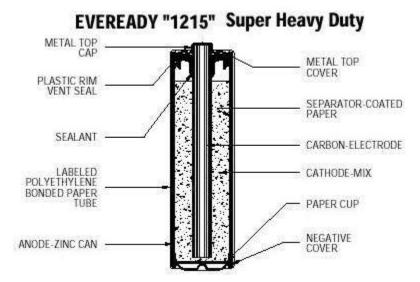
Cathodes are a mixture of manganese dioxide, carbon conductor and electrolyte.
