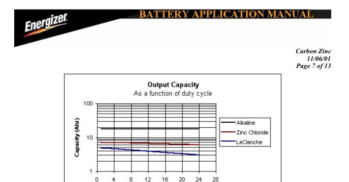
The electrochemical inputs of cylindrical D size batteries typically are in a ratio of 2:3:5 for LeClanche, Zinc Chloride and Alkaline respectively. The differences in efficiency and rate sensitivity between the three systems cause variations in actual output in simulated typical applications as shown in the following table and graph:
