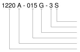
Pressure Tubes (L = Long, S = Short, N = None) Lead Configuration (1,3 - See Dimensions Diagram) Type (G= Gage, A = Absolute, D = Differential) Pressure Range Grade Model
