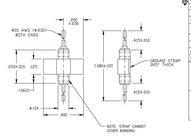
LEAD FINISH: SOLDER GROUND STRAP: FINISH: SILVER CAPACITANCE pF 12,000pF GMV TEMP, RANGE -55°C TO 125°C CURRENT 10 AMP DC 85°C, 100 VDC WORKING VOLTAGE 125°C, 70 VDC D.C. RESISTANCE .01 ohms INSERTION LOSS PER MIL-STD-2201 (NO LOAD) FREQ.(MHz) 100 1GHz 10 25 65 LIMITED (dB) 70
