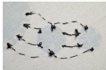
Stitching the sensor into a project is easy-- just line up the sensor so its adjacent to the SDA/SCL pins on Flora or another I2C sensor, and stitch the four connections with conductive thread. This is covered in more detail in the Flora Accelerometer (http://adafru.it/aYS) guide and our Conductive Thread (http://adafru.it/aVx) guide.
