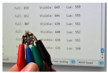
Open the serial monitor (the upper right button in the Arduino IDE) and watch the sensor values pour in.
