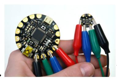
To test the sensor before sewing it into a project, use alligator clips to
