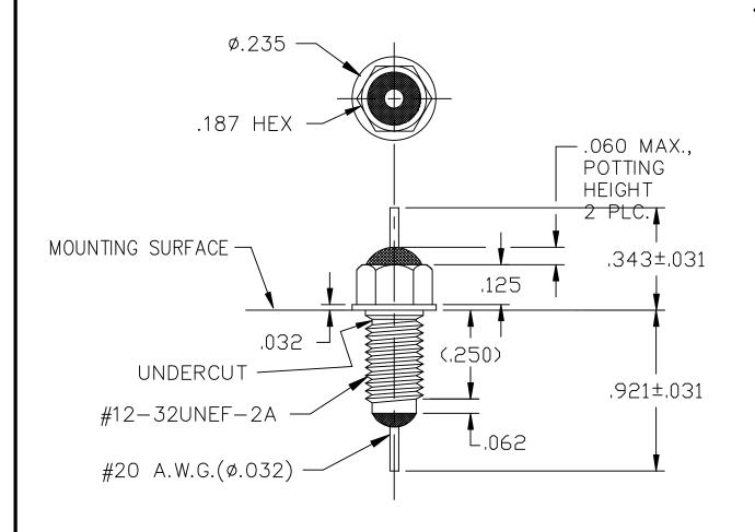
BUSHING FINISH: SILVER LEAD FINISH: SILVER CAPACITANCE 3000pF MIN. TEMP, RANGE -55°C TD +125°C **CURRENT** 10 AMPS 85°C 350 VDC WORKING VOLTAGE 125°C 200 VDC DC .01 DHMS MAX. RESISTANCE IL=PER MIL-STD-220, NO LOAD FREQ. MHz I.L. (db) 10 50 N/A 45 100
