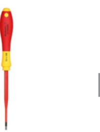
VDE insulated screwdriver sets, for working on live parts up to 1000 V AC and 1500 V DC, DIN EN 60900. IEC 900. Each piece is "GS" safety tested. Blade made from fully hardened, high-alloy chromium-vanadiummolybdenum steel, gun-metal finish.
