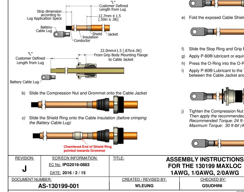
d) Crimp the Battery Cable Lug onto the Conductor
