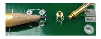
Due to their miniature size, MMCX Connectors are ideal for high density applications requiring a very small RF interconnect.
