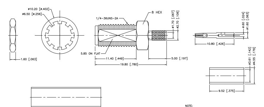
1. CRIMPED FERRULE HEX CRIMP SIZE .151" [3.83] 2. CONTACT PIN TO SOLDER.
