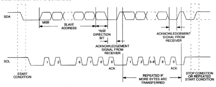
Depending upon the state of the  $R/\overline{W}$  bit, two types of data transfer are possible:
