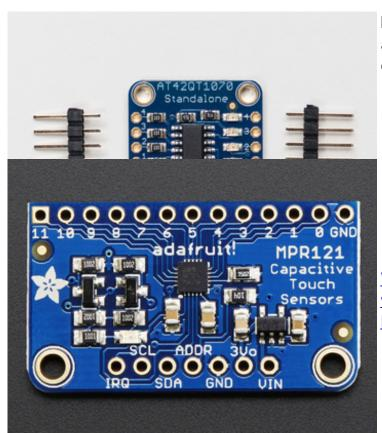
breakout. There are 5 pins for attaching wires to up to 5 external sensor pads.
