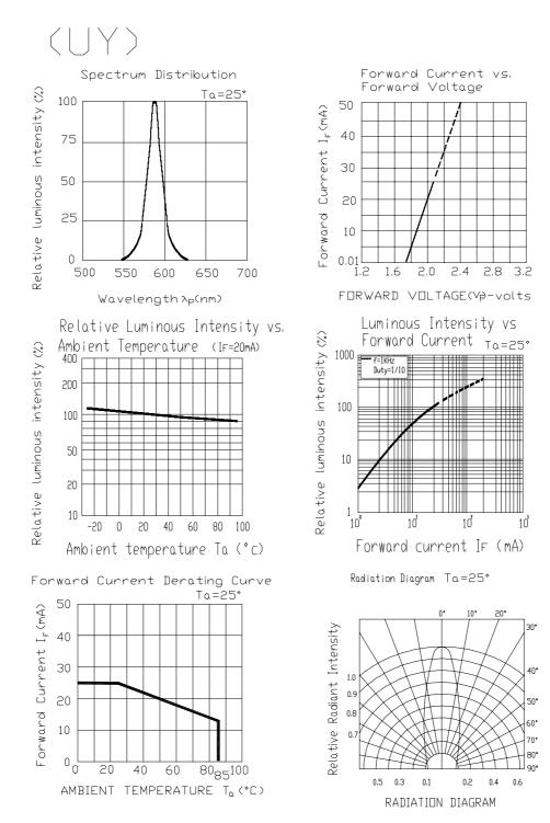
Typical Electro-Optical Characteristic Curves:
