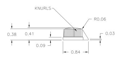
USE #28 DRILL (0.140), #8-32 TAP, #8-32 X 1/4 LG. CUP POINTED, SLOTTED TYPE, SET SCREW 10357 (1).
