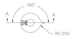
USE #28 DRILL (0.140), #8-32 TAP, #8-32 X 3/16 LG. CUP POINTED, SLOTED TYPE, SET SCREW 10328 (1).
