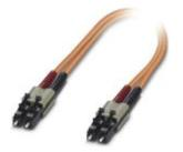
Assembled FO cable, zip cord cable, multi-mode fiberglass 50/125  $\mu$ m, OM2, plug: LC/LC, degree of protection: IP20, for installation in cable ducts or control cabinets, length: 2 m
