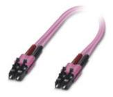
Assembled FO cable, zip cord cable, multi-mode fiberglass 50/125  $\mu$ m, OM4, plug: LC/LC, degree of protection: IP20, for installation in cable ducts or control cabinets, length: 2 m
