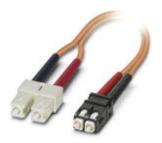
Assembled FO cable, zip cord cable, multi-mode fiberglass 50/125 µm, OM2, plug: SC duplex/SCRJ, degree of protection: IP20, for installation in cable ducts or control cabinets, length: 2 m
