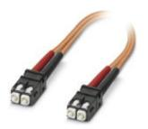
Assembled FO cable, zip cord cable, multi-mode fiberglass 50/125  $\mu$ m, OM2, plug: SCRJ/SCRJ, degree of protection: IP20, for installation in cable ducts or control cabinets, length: 2 m
