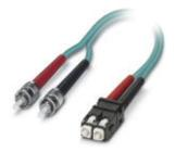
Assembled FO cable, zip cord cable, multi-mode fiberglass  $50/125 \,\mu m$ , OM3, plug: B-FOC (ST)/SC-RJ, degree of protection: IP20, for installation in cable ducts or control cabinets, length: 2 m
