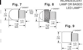
Material & Finish: Base - Black Nickel Plated Brass, Cap - High Impact Plastic; Polycarbonate with Black Nickel Bezel (Fig. 8)
