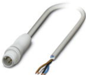
Sensor/Actuator cable, 4-position, PP-EPDM halogen-free, Gray RAL 7035, Plug straight M12, A-coded, on Free cable end, Cable length: 1.5 m, Hygienic design, with plastic knurl
