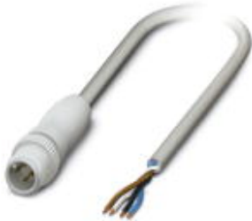
Sensor/Actuator cable, 4-position, PP-EPDM halogen-free, Gray RAL 7035, Plug straight M12, A-coded, on Free cable end, Cable length: 10 m, Hygienic design, with plastic knurl
