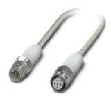
Sensor/Actuator cable, 5-position, PP-EPDM halogen-free, Gray RAL 7035, Plug straight M12, A-coded, on Socket straight M12, A-coded, Cable length: 0.3 m, Hygienic design, With high-grade steel knurl
