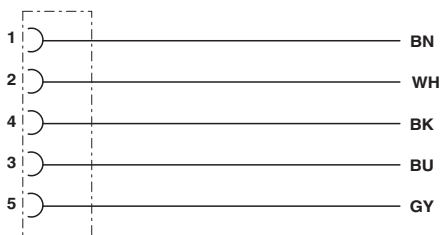
Contact assignment of the M12 socket
