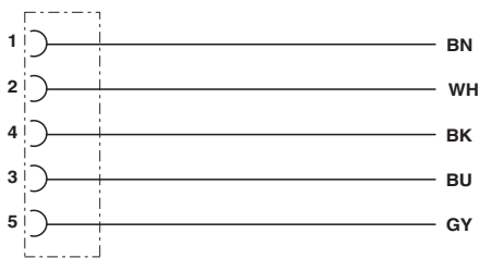
Contact assignment of the M12 socket
