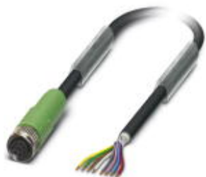
Sensor/actuator cable, 8-position, PUR halogen-free, black RAL 9005, shielded, free cable end, on Socket straight M8, cable length: 1.5 m
