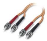
Assembled FO cable, zip cord cable, multi-mode fiberglass 50/125  $\mu$ m, OM2, plug: B-FOC (ST)/B-FOC (ST), degree of protection: IP20, for installation in cable ducts or control cabinets, length: 2 m
