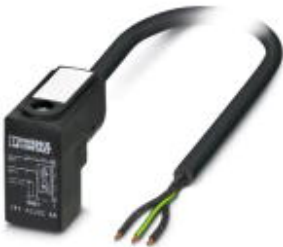
Sensor/Actuator cable, 3-position, PVC, Black RAL 9005, Free cable end, on C valve plug (8 mm), with 1 LED, connected with Z diode, Cable length: 10 m
