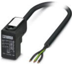
Sensor/Actuator cable, 3-position, PVC, Black RAL 9005, Free cable end, on CI valve plug (9.4 mm), with 1 LED, connected with Z diode, Cable length: 2 m
