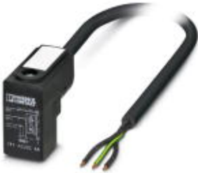
Sensor/Actuator cable, 3-position, PVC, Black RAL 9005, Free cable end, on CI valve plug (9.4 mm), with 1 LED, connected with Z diode, Cable length: 5 m
