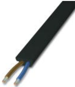
AS-Interface PVC flat conductor with UL in black, for additional power supply, 2 x 1.5 mm 2 , 1000 m on an one-way drum
