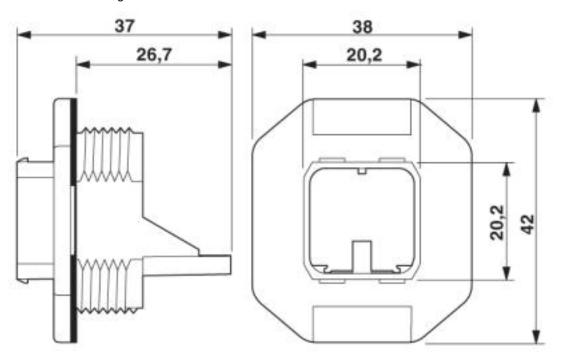
Push-Pull panel mounting frame, Freenet system, IP67
