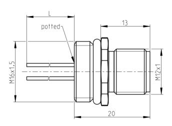
All specified data refers to the mounted M12 installation plugs ≥ IP54 and requires that the connector pair be correctly plugged and locked. Influences from wires, cables or PCB mounting are also to be taken into consideration.
