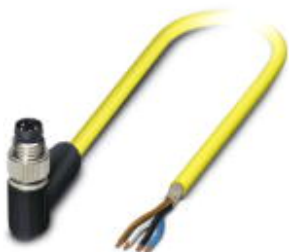
Sensor/Actuator cable, 4-position, PVC, yellow, shielded, Plug angled M8, on free cable end, Cable length: 5 m
