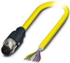
Sensor/Actuator cable, 8-position, PVC, yellow, shielded, Plug straight M12 SPEEDCON, A-coded, on free cable end, Cable length: 10 m
