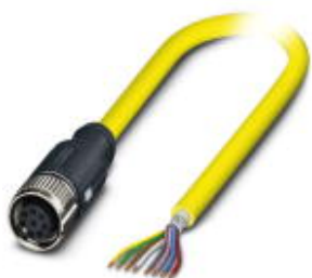
Sensor/Actuator cable, 8-position, PVC, yellow, shielded, free cable end, on Socket straight M12 SPEEDCON, A-coded, Cable length: 2 m
