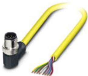
Sensor/Actuator cable, 8-position, PVC, yellow, Plug angled M12 SPEEDCON, A-coded, on free cable end, Cable length: 5 m
