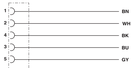
Contact assignment of the M12 socket
