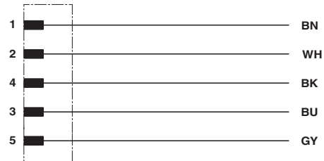
Contact assignment of the M12 plug
