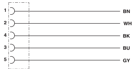
Contact assignment of the M12 sockets
