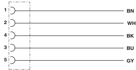
Contact assignment of the M12 sockets
