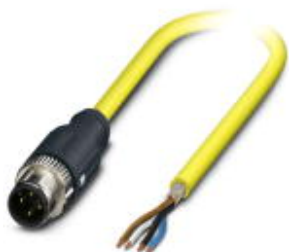
Sensor/Actuator cable, 4-position, PVC, yellow, shielded, Plug straight M12 SPEEDCON, A-coded, on free cable end, Cable length: 10 m
