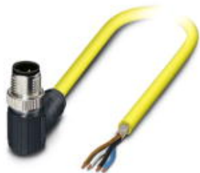
Sensor/Actuator cable, 4-position, PVC, yellow, shielded, Plug angled M12 SPEEDCON, A-coded, on free cable end, Cable length: 10 m
