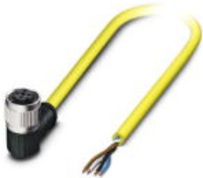
Sensor/Actuator cable, 4-position, PVC, yellow, free cable end, on Socket angled M12 SPEEDCON, A-coded, Cable length: 2 m
