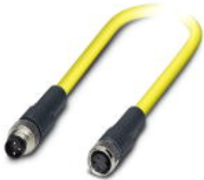
Sensor/Actuator cable, 3-position, PVC, yellow, Plug straight M8, on Socket straight M8, Cable length: 1.5 m
