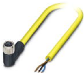
Sensor/Actuator cable, 3-position, PVC, yellow, free cable end, on Socket angled M8, Cable length: 2 m
