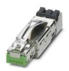
RJ45 connector, Degree of protection: IP20, Number of positions: 8, 10 Gbps, Material: Zinc die-cast, Connection method: IDC, Connection cross section: AWG 26-24, Cable exit: straight, High degree of resistance to vibration; 360° shielding; one-piece design; special tool-free assembly
